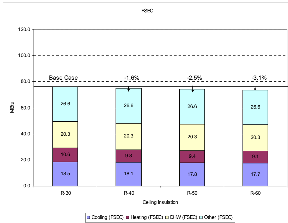
Figure 12. Ceiling insulation (FSEC) with the duct leakage.
